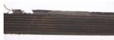
Typical Belt Wear
