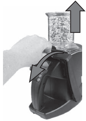
Figure 3. Pull level arm forward. Lift hopper up.
