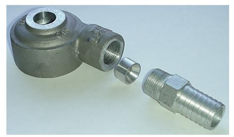
Then insert the bushing as shown in the photo below with the angle portion of the bushing facing the hose barb and replace the inlet hose barb and tighten.
