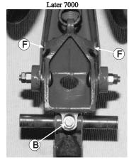
furrow if necessary. Note that it may be necessary to grind some material off of the support lugs (F) to utilize this adjustment. It may also be necessary to grind two corners off the carriage bolt neck to allow full adjustment.
