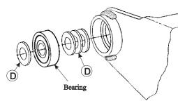
Note: The inside diameter of the bearing housing has been machined to provide approximately .015" clearance with the bearing outer race. This is to allow for some misalignment between the bearings. The bearing outer race will not slip in the housing because the friction between the balls and races is very low in comparison to that between the outer race and housing.
