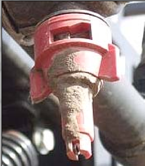
Plugged Air Hole in Normal Conditions
