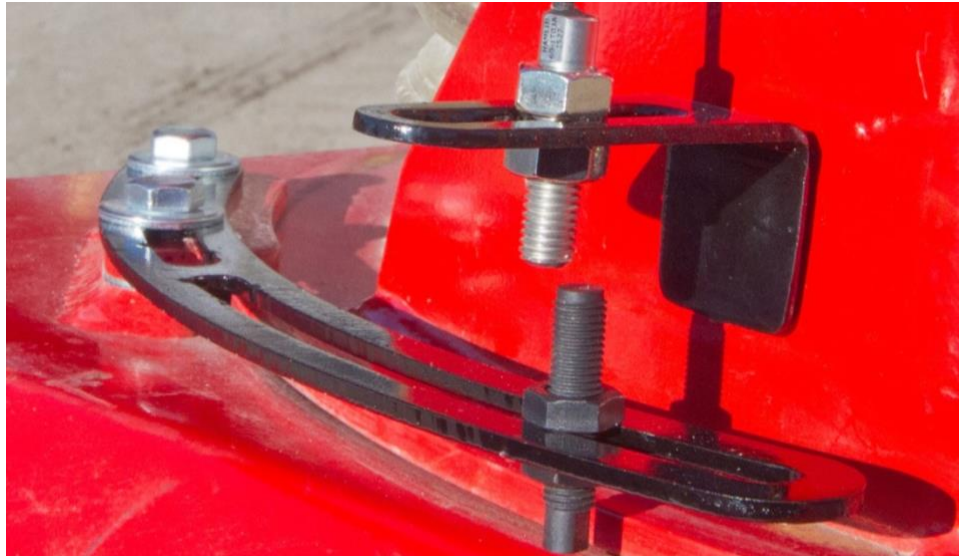
Limit stop sensor and limit stop adjusted properly
