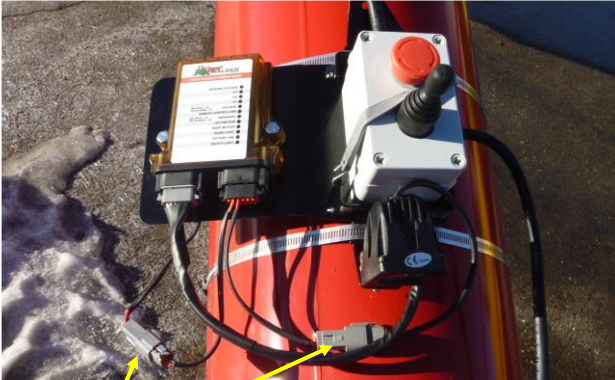
H1 shown with beeper and light cables attached.
