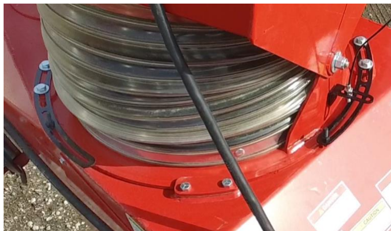
Both limit stop brackets installed on auger boot.
