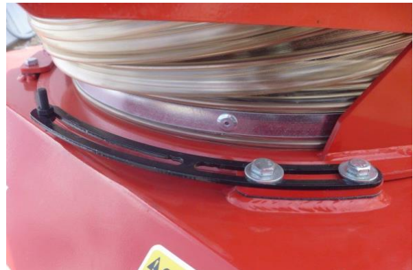
Limit stop bracket installed on spout head retainer
