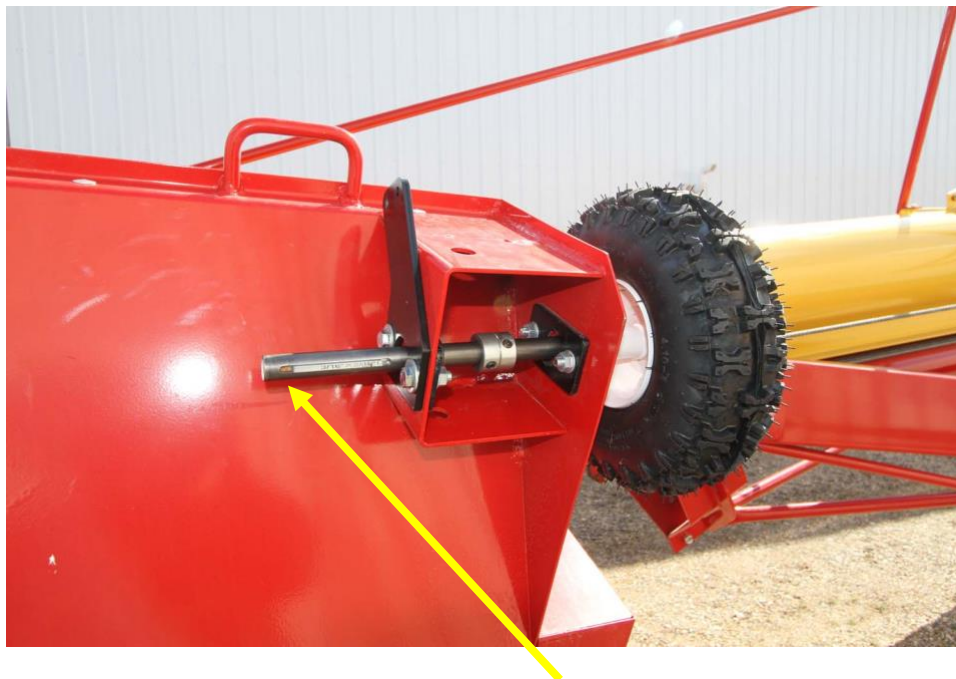
Tire installed on outside of hopper. Note the keyway for the motor; it is NOT cut to the end of the shaft. Leave approximately \frac{1}{2} " – 1" of clearance between the tire and the hopper.
