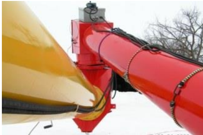
Swing hopper tube with 6" of clearance between main auger tube.
