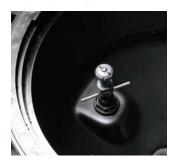
ProClean™ bottle rinse allows operator to triple rinse chemical containers on-site for legal disposal.
