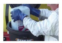
ProClean™ bottle rinse allows operator to triple rinse chemical containers on-site for legal disposal.
