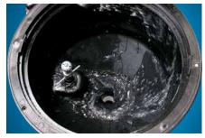
CycloRinse<sup>™</sup> system provides premium cleaning and meltdown of flowable powders, such as AMS, with an open lid for continuous-fill operation.
