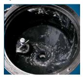
CycloRinse™ system provides premium cleaning and meltdown of flowable powders, such as AMS, with an open lid for continuous-fill operation.
