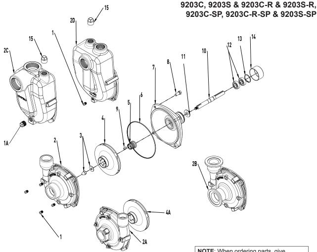
Silicon Carbide Seal Kit No. 3430-0589 consists of:
